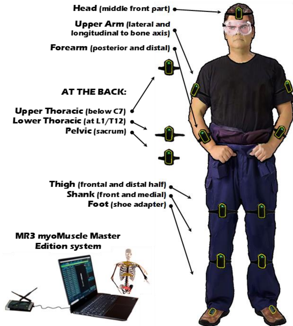
Figure 1. The measurement set-up with the computer workstation and locations of the sensors on the worker's body.
