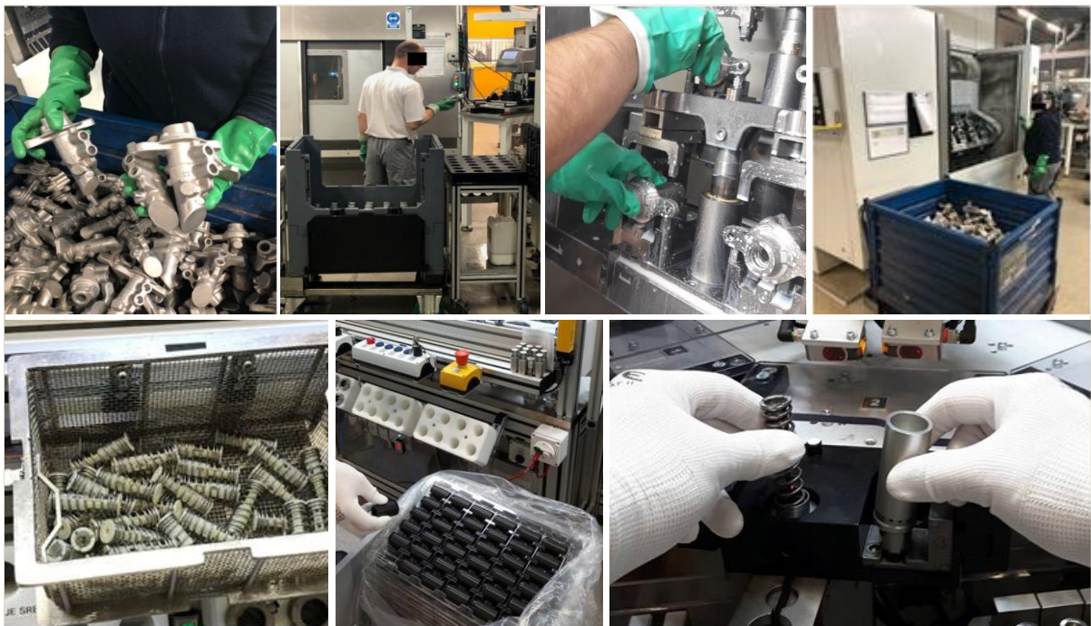
Figure 2. A sequence of production activities at the machining (above) and assembly workstation (below). [Used with permission]
