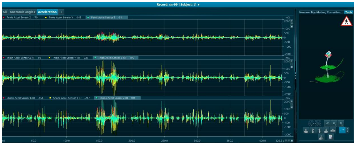
Figure 4. Acceleration values (3D signals from triaxial accelerometers).
