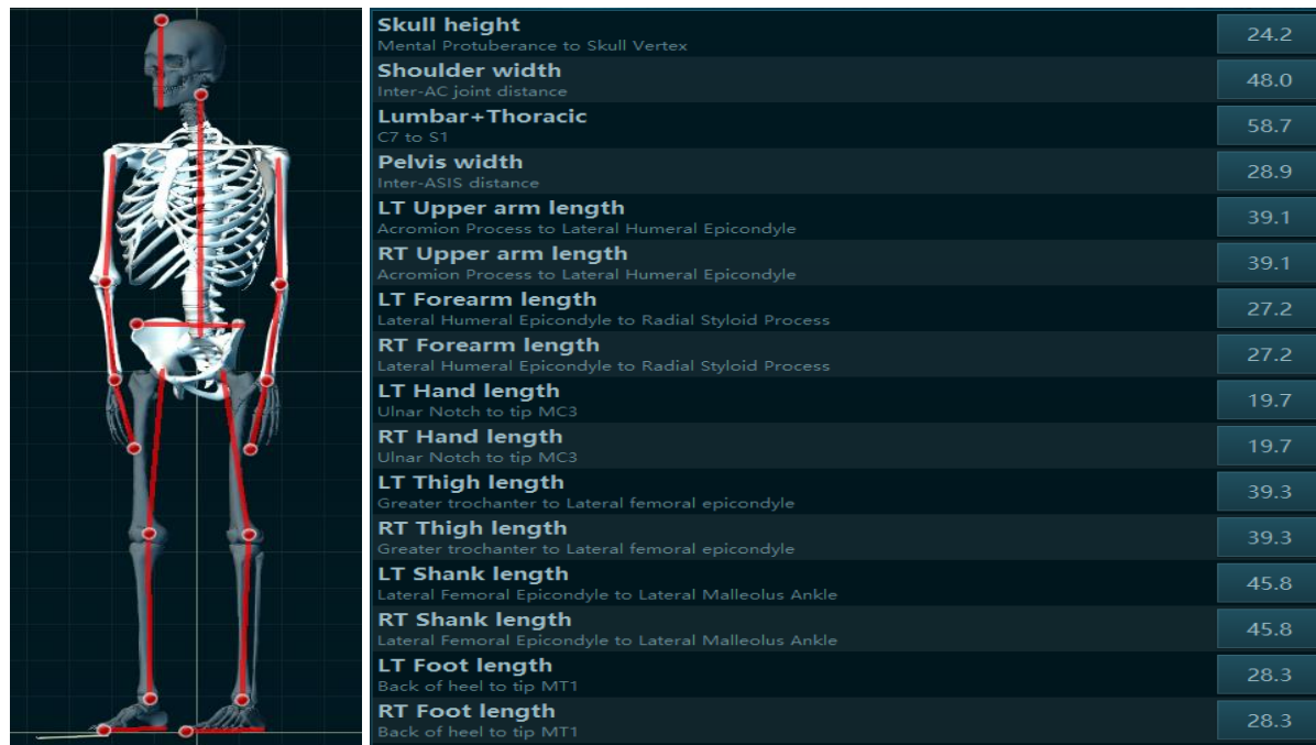
Figure 5. The three degree and 16 body parts model for the determination of segment mass and length.
